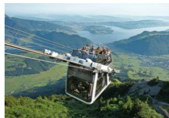
Open deck aerial cable car
