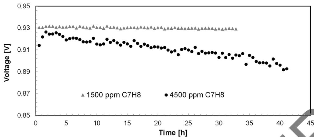
Figure 5. Polarization over time at 800°C, 0.25 A/cm<sup>2</sup>. At 4500 ppm, the degradation rate is 70 mV/100h.
