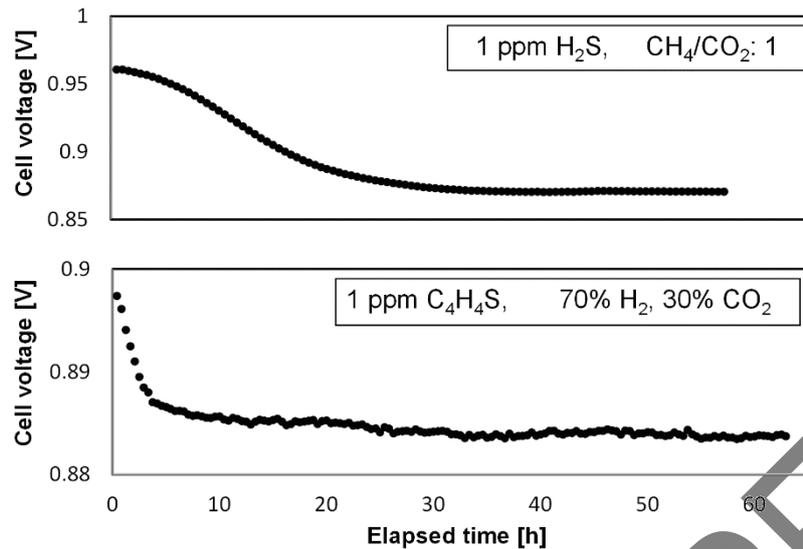
Figure 2. Sulfur poisoning. Polarization over time at 750 °C under 0.25 A/cm<sup>2</sup>. SOLIDpower cell.
