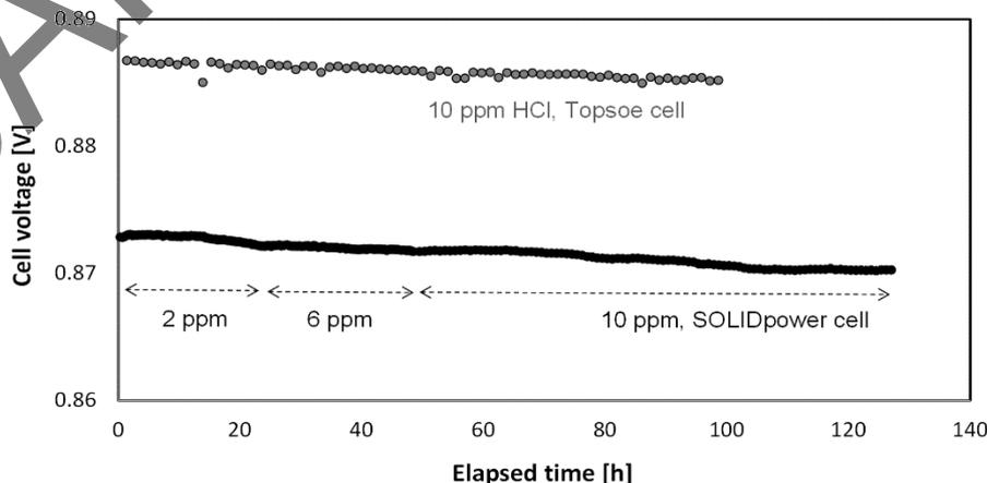
Figure 3. HCl poisoning at concentrations up to 10 ppm. Polarization over time at 750 °C under 0.25 A/cm<sup>2</sup>.
