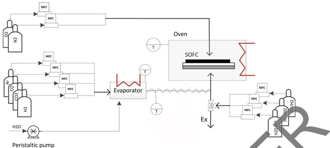
Figure 1. Scheme of SOFC single cell test rig for the poisoning experiments.
